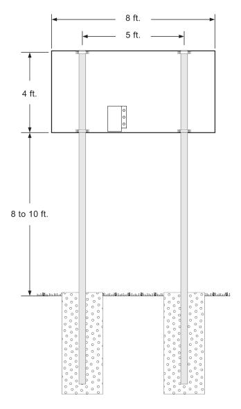
Once you have verified the positions of the posts and the size of the footings, you are ready to dig your holes, pour your concrete, and set your posts. There are several techniques for ensuring proper alignment of the posts. Typically installers will construct a temporary wooden support frame to hold each post in place while the concrete sets. Having plumb posts in the proper position is the key to a smooth mechanical installation.
